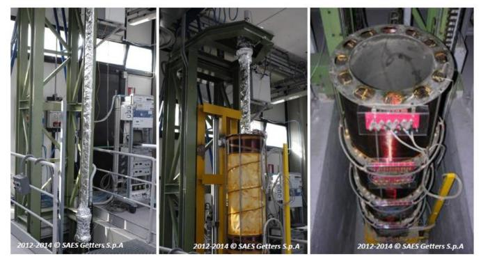
One of the SAES sputtering systems for NEG coating, capable to coat up to 6.5 meter long chambers with a 2m height coil.
