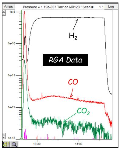
This activation of a SAES' CapaciTorr D100 pump shows typical behavior. (The pump was previously saturated with CO gas, after a 24-hr pumping.)
