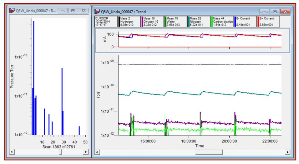
RGA data showed hydrogen being the dominant gas, with trace of other gases (probably produced by RGA filament)
