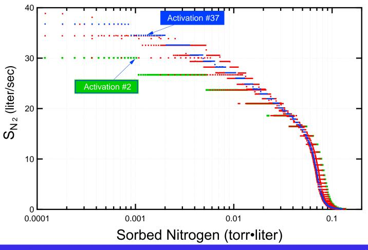
Measured N<sub>2</sub> pumping on a CapaciTorr D100 pump with repeated activation/saturation cycles w/o venting
