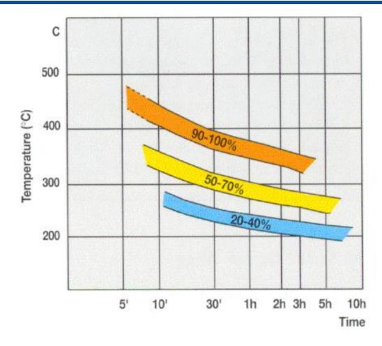
Fig. 1. Activation conditions and gettering efficiency of St 707
